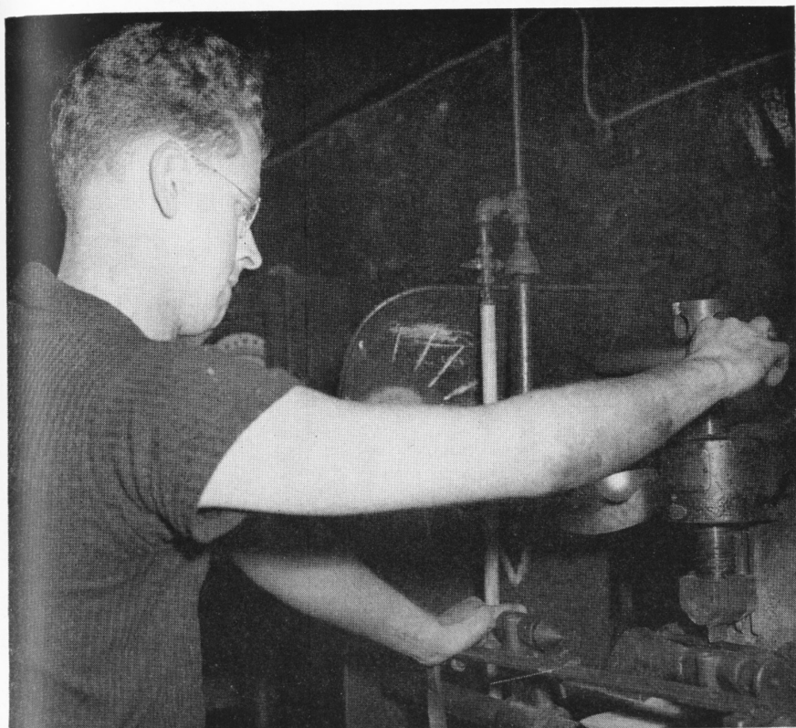
Here's John Engratt at the straightening machine. Sometimes it's necessary to straighten tools after they have been through the hardening and tempering process. Heat is being applied to the punch with a torch at the same time pressure is applied with a screw. A perfectly straight punch will be handed over to the Grinding Room.
